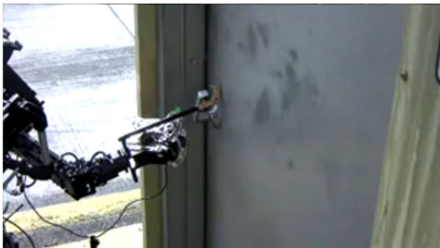
Figure 18. THOR-OP used a hook to hold and rotate the handle for the door task. Almost 80 degrees was required to open the door, which was unexpected and harder than our testing setup, which only required 60 degrees.
