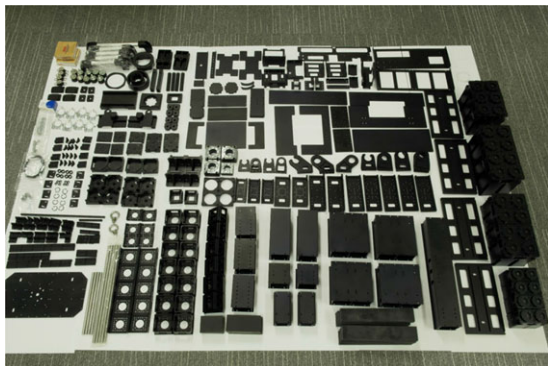
Figure 4. The structural components for a single THOR-OP robot use standardized dimensions.
