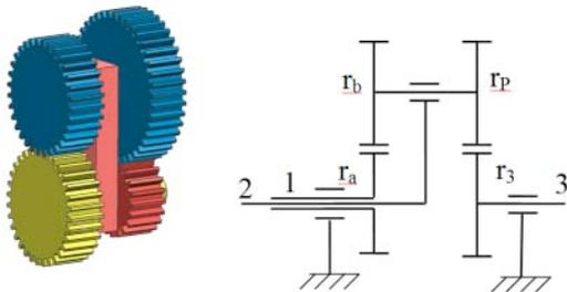
**Figure 5: Planet gearset representative of the Cam-based IVT.**
