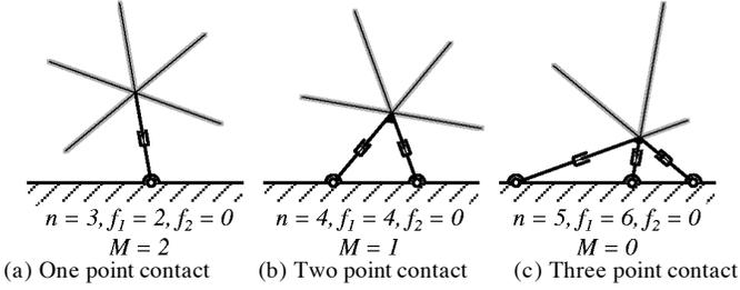
Fig. 4 Kinematic diagram of a single actuated spoke wheel and its degrees of freedom for different modes.
