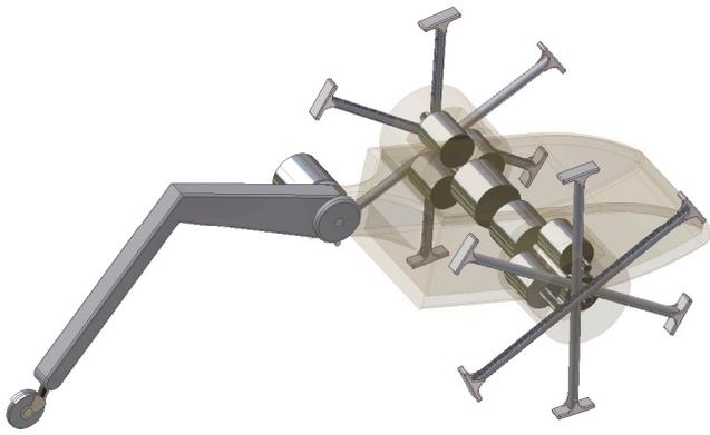
Fig. 6 IMPASS with two actuated spoke wheels and an articulated tail.
