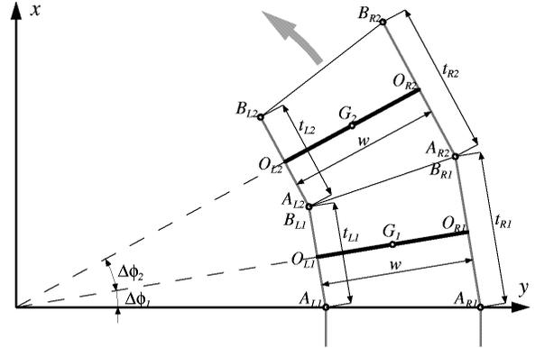
Fig. 5 Discrete turning by changing the spokes length for the one-point contact mode.
