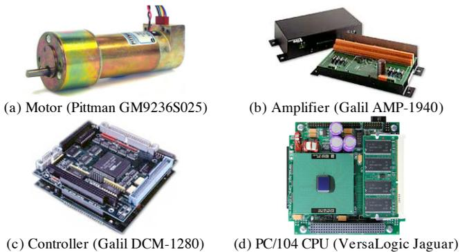
Fig. 6 Electronic components.
