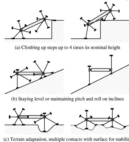
Fig. 1 Some examples of the mobility and terrain adaptability of IMPASS.
