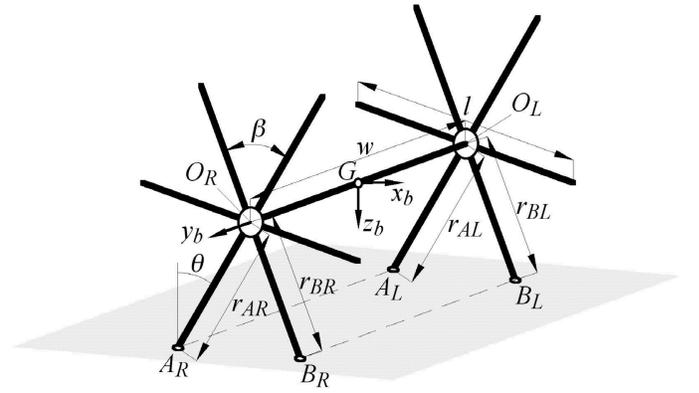
Fig. 3 Two actuated spoke wheels with a single axle.
