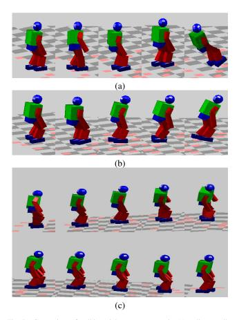
Fig. 5. Comparison of walking trials on uneven terrain. (a) walk controller with push recovery controller (b) walk controller with surface learning (c) walk controller with both surface learning and push recovery control.
