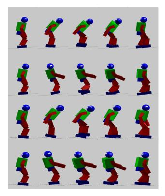
Fig. 4. Responses of learned push recovery controller for external perturbation on inclined and declined surface.
