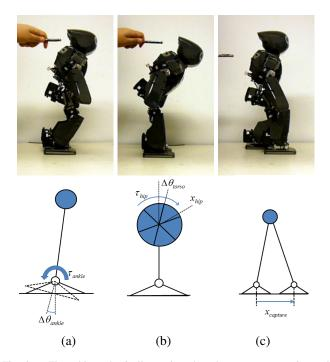
Three biomechanically motivated push recovery strategies and corresponding controller for position-controlled robot based on simplified model. (a) Ankle strategy that applies control torque on ankle joints. (b) Hip strategy which uses angular acceleration of torso and limbs to apply counteractive ground reaction force (c) Step strategy which moves center of pressure to a new position.
