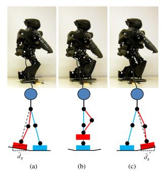
Walk controller for uneven terrain. (a) The swing foot starts at ground position with distance variable  $\vec{d}_R$ . (b) The foot pose follows the computed trajectory during the early phase of the step, and the swing leg becomes compliant during the latter part of the step. (c) After the footfall, the swing leg stiffens and new disturbance variable  $\vec{d_R}'$  is measured to keep the torso upright at the next step.
