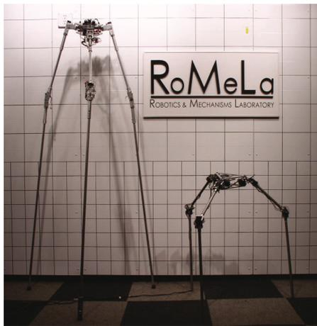
**Fig. 1.** STriDER 2.0 prototype on right of its predecessor, STriDER
