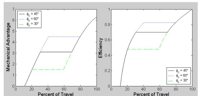
Figure 7. MECHANICAL ADVANTAGE AND EFFICIENCY FOR A COMPOSITE CROSS-SECTION CST WITH VARYING SLOPE ANGLES.
