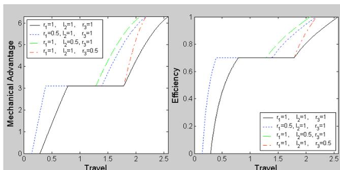
Figure 8. MECHANICAL ADVANTAGE AND EFFICIENCY FOR A COMPOSITE CROSS-SECTION CST WITH VARYING GEOMETRY.
