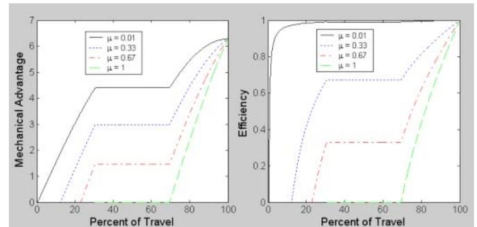
Figure 6. MECHANICAL ADVANTAGE AND EFFICIENCY FOR A COMPOSITE CROSS-SECTION CST WITH VARYING FRICTION COEFFICIENTS.
