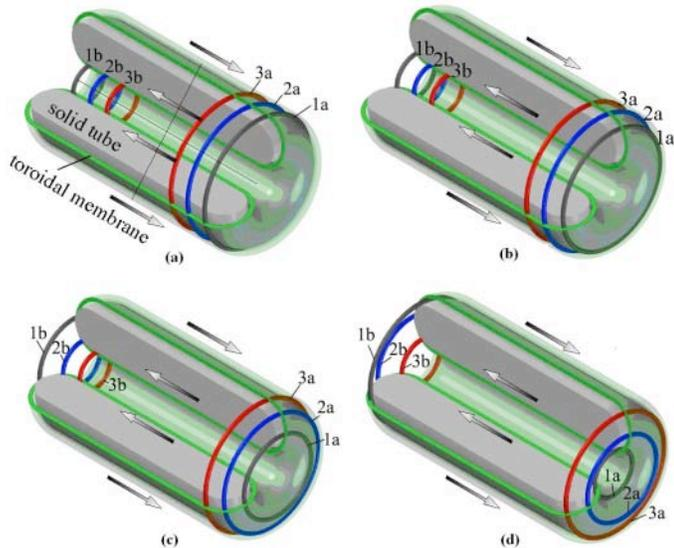
Figure 1. EVERTING MOTION GENERATED BY THE CONTRACTING (1a, 2a, 3a) AND EXPANDING (1b, 2b, 3b) ACTUATOR RINGS FOR THE CONCENTRIC SOLID TUBE WSL MODEL.
