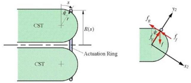
(a) Cross section of CST with a contracting ring (b) Free body diagram
