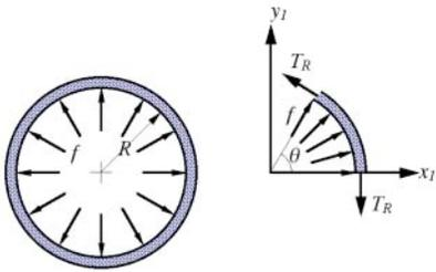
Figure 2. FREE BODY DIAGRAM OF A CONTRACTING RING ACTUATOR
