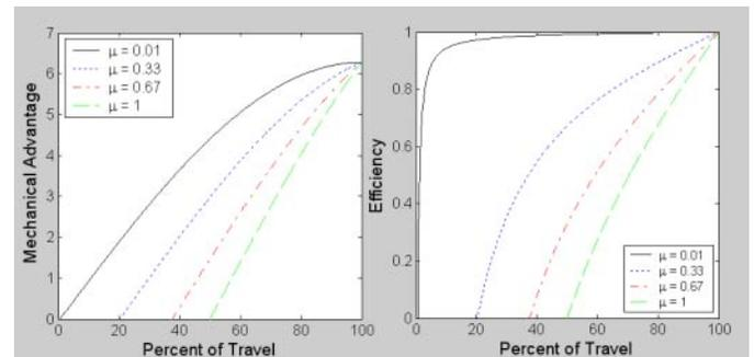
Figure 4. MECHANICAL ADVANTAGE AND EFFICIENCY VERSUS PERCENT OF TRAVEL FOR A CIRCULAR CROSS-SECTION CST WITH VARYING FRICTION COEFFICIENTS.
