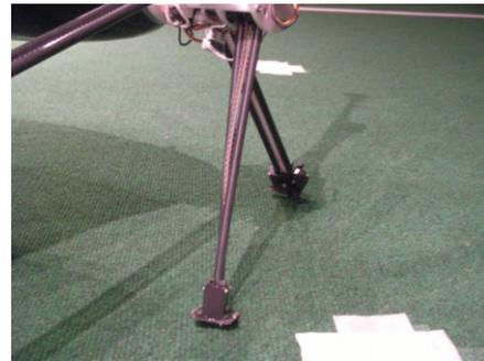
**Figure.13** Spoke twisting
