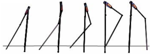
Figure 6. Simplification to the four link STriDER model that allowed for the application of the self-excited controller
