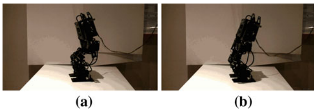
Fig. 2 Video stills of a robot leaning back and forth to maintain stability by moving the COM location in the X -direction
