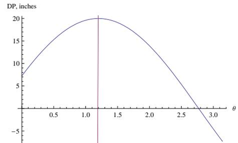
Figure 11. THE DP IS SHOWN FOR WHEN THE BACK SPOKE IS AT  $l_{min}$  AND THE FRONT SPOKE IS AT  $l_{max}$ , AND REACHES THE MAXIMUM DP AT  $\theta = \frac{2*\pi}{3} = 120^\circ$ .
