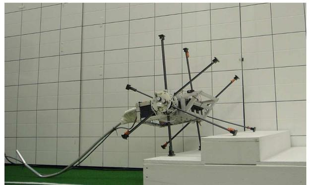
Figure 1. A PROTOTYPE OF THE IMPASS ACTUATED SPOKE WHEEL PLATFORM HAS BEEN DEVELOPED FOR MOTION PLANNING RESEARCH.
