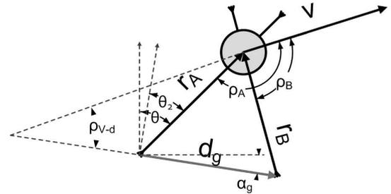
Figure 7. IMPASS SHOWN IN THE TWO-POINT CONTACT CONFIGURATION. TRANSITIONS FOR THE ONE-POINT CONTACT GAIT ARE DESCRIBED USING THE SWITCHING ANGLES,  $\theta$  AND  $\theta_2$ .
