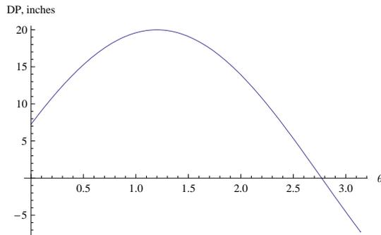
Figure 10. THE DESCENDING POTENTIAL (DP) IS SHOWN FOR EQUAL LENGTHS OF THE FRONT AND BACK SPOKES. THE MAXIMUM DP IS REACHED AT  $\theta = \frac{2*\pi}{3} = 120^\circ$ .
