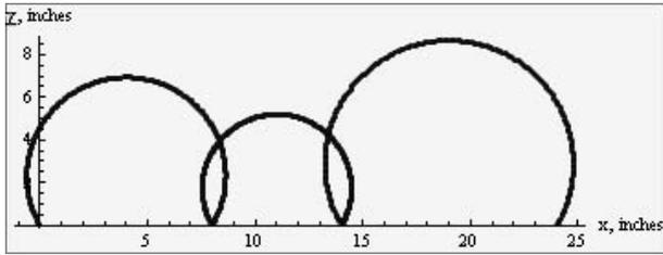
Figure 5. THE HUB CENTER PATHS FOR THREE CONSECUTIVE STEPS WITH CONTACT POINTS AT 0, 8, 14 AND 24. THE POINTS OF INTERSECTION OF THE ARCS ARE WHERE STEP TRANSITIONS CAN OCCUR.
