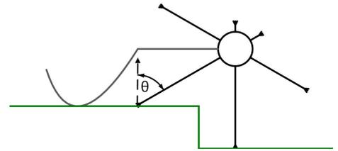
Figure 9. IMPASS DESCENDING AN OBSTACLE WITH  $\theta = 60^\circ$ .
