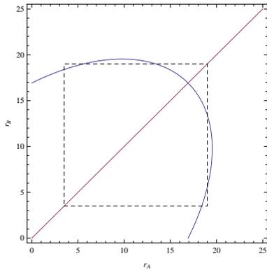
Figure 6. THIS GRAPH PLOTS THE LENGTH OF THE BACK SPOKE AGAINST THE LENGTH OF THE FRONT SPOKE DURING A STEP OF 17 INCHES. A DASHED BOX HAS BEEN INCLUDED WHICH SHOWS THE MAXIMUM AND MINIMUM SPOKE LENGTHS [7].
