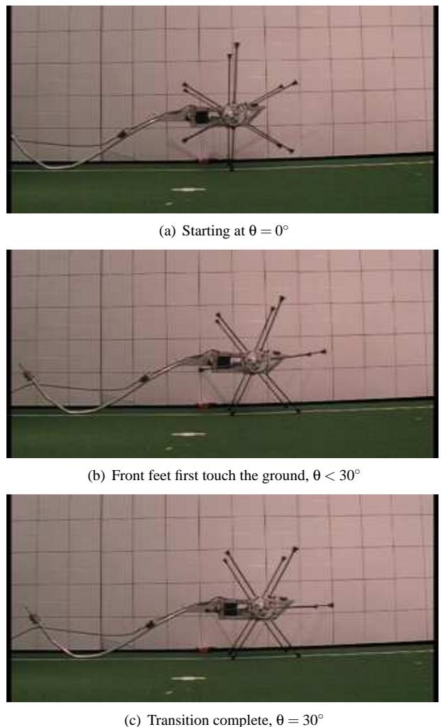
Figure 13. TESTING OF THE DEFAULT TRANSITION. THE FRONT SPOKES TOUCH THE GROUND BEFORE  $\theta = 30^\circ$  DUE TO COMPLIANCE IN THE SPOKES AND BACKLASH IN THE HUB GEAR TRAIN.
