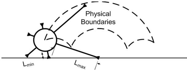
Figure 4. THE PHYSICAL BOUNDARIES OF THE HUB CENTER ARE SHOWN FOR THE ONE-POINT CONTACT GAIT, DETERMINED BY THE MINIMUM AND MAXIMUM SPOKE LENGTHS,  $L_{min}$  and  $L_{max}$ .
