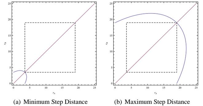
Figure 8. THE SPOKE LENGTHS,  $\vec{r}_A$  and  $\vec{r}_B$ , ARE PLOTTED AGAINST EACH OTHER FOR THE MINIMUM AND MAXIMUM STEP LENGTHS [7].
