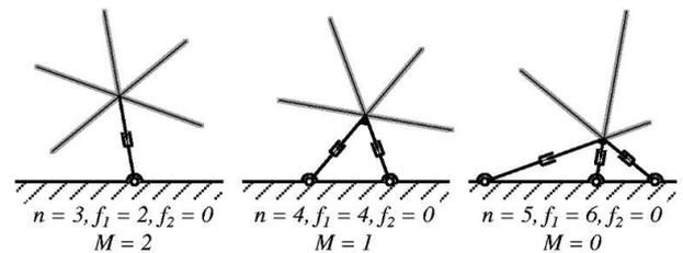
Figure 3. A SINGLE ACTUATED RIMLESS WHEEL CAN CONTACT THE GROUND IN THREE WAYS, RESULTING IN TWO, ONE, OR ZERO DEGREES OF FREEDOM [5].
