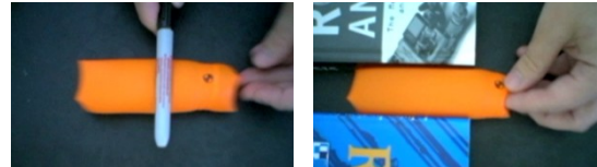
Fig.2. Fluid filled toroid model demonstrating the ability to squeeze under obstacles and through holes.
