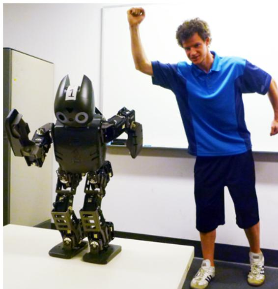
Fig. 1. The DARwIn-OP robot imitating the full body behavior of human operator in real time
