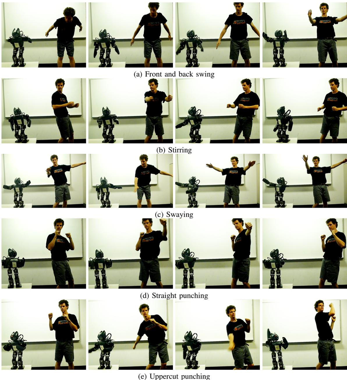
Fig. 7. The real-time imitation of various full-body human motions by the DARwIn-OP robot.
