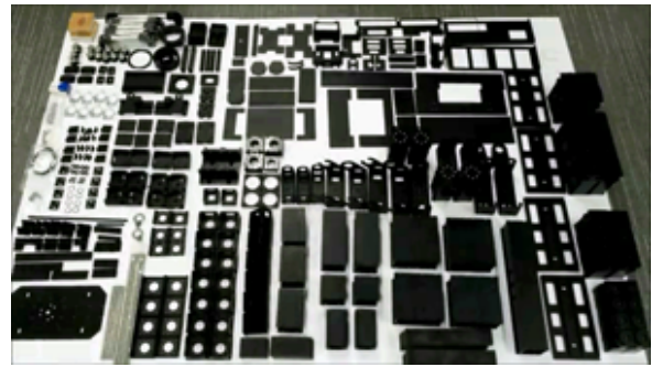
Fig. 3. The structural components for a single THOR-OP robot use standardized dimensions.
