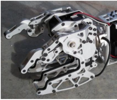
Fig. 5. The gripper for the DRC Trials consisted of two under actuated fingers to wrap around an object, and a rigid palm to give support.
